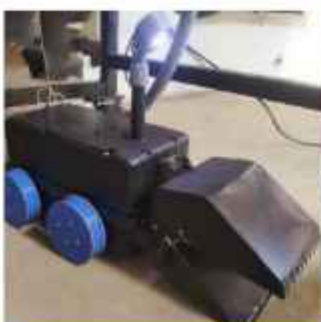
PIPE BOT FOR CLEANING
